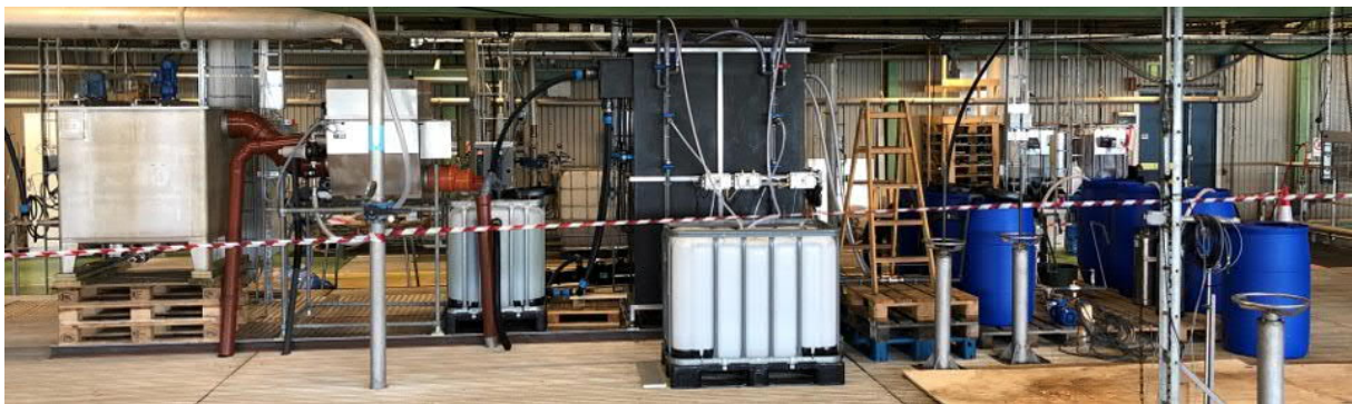
Figure 4. DMF pilot plant including coagulation/flocculation tank (left side), drum sieve, retention tank and membrane unit (middle, black)
